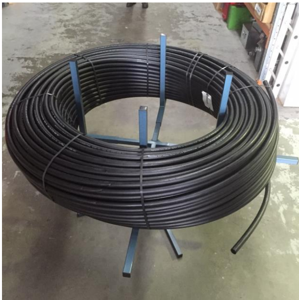
Loaded with a 660M Coil of 32mm Subduct
