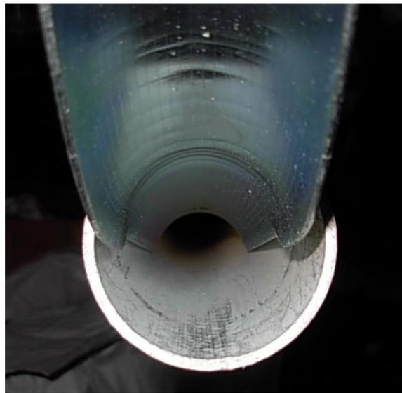
**Incorrect insertion** – End view shows obstructed cable entry which may impede installation or cause damage to the cable
