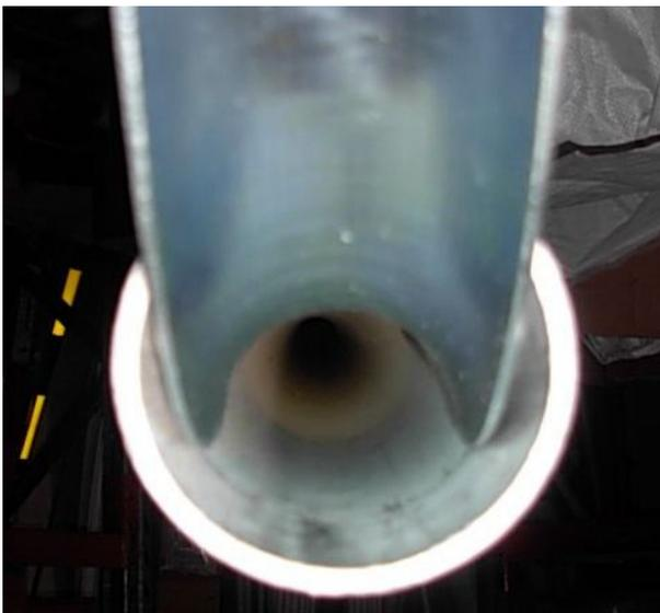
**Correct insertion** – End view shows unobstructed cable entry providing maximum working area
